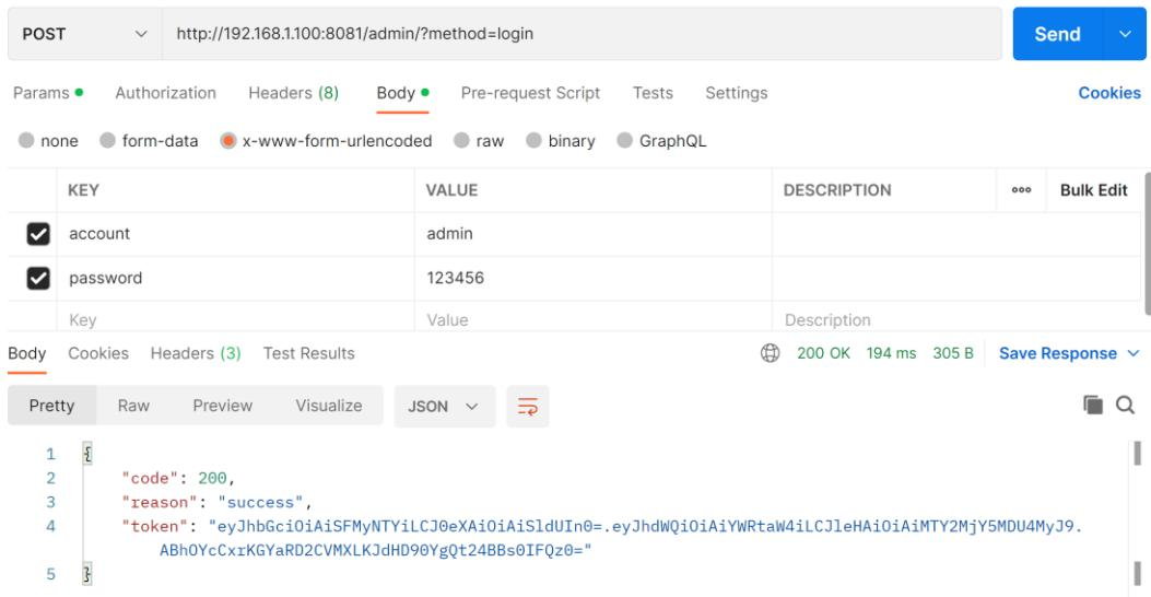
The screenshot shows a Postman interface with a POST request to `http://192.168.1.100:8081/admin/?method=login`. The 'Body' tab is selected, showing the data type as 'x-www-form-urlencoded'. There are two fields: 'account' with value 'admin' and 'password' with value '123456'. The response status is 200 OK with a duration of 194 ms and a size of 305 B.
